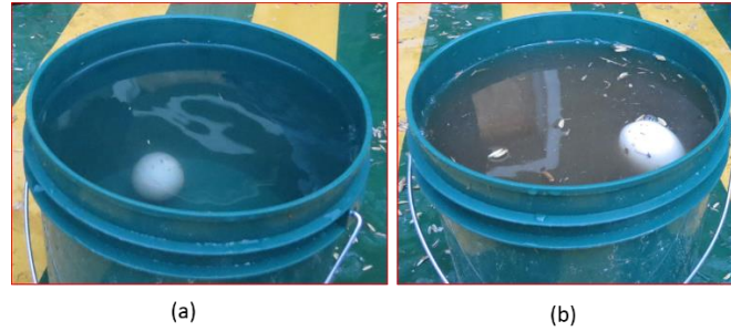
Figure 1: (a) Submerged egg before adding salt (b) A floating egg after adding salt
