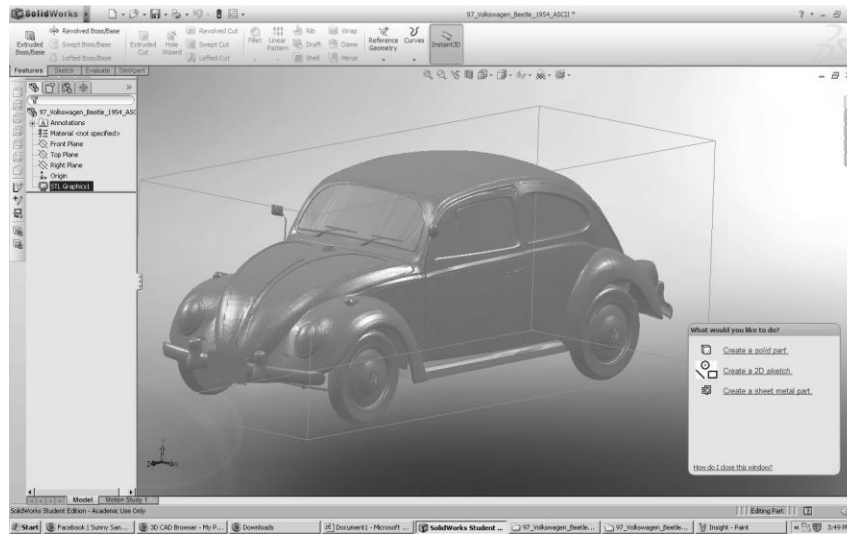
Figure 7: CAD version of the study vehicle model in a CFD Add-on environment
